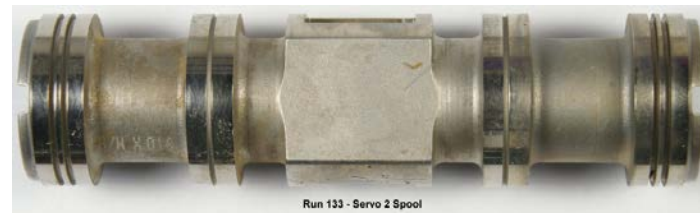
Figure 46 – Comparison of Start and End Program Servo Valve Spools, EDTST-Mode, Baseline and Additized Fuels
