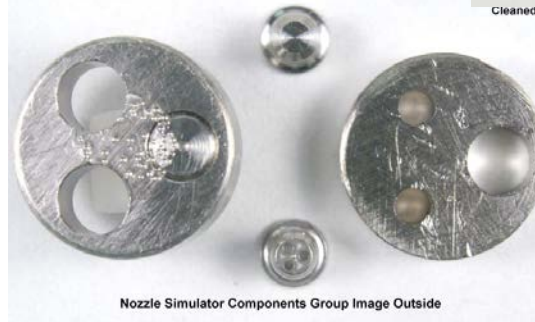
Figure 39 – Comparison of Nozzle Simulator Components, EDTST-Mode, Baseline and Additized Fuels
