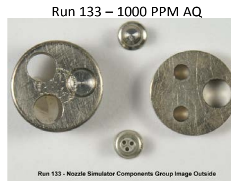
Figure 47 – Comparison of Start and End Program Nozzle Simulator Components, EDTST-Mode, Baseline and Additized Fuels
