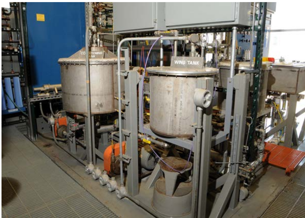
Figure 2 - Conditioning Tank (Left) and Wing Tank (Right)
