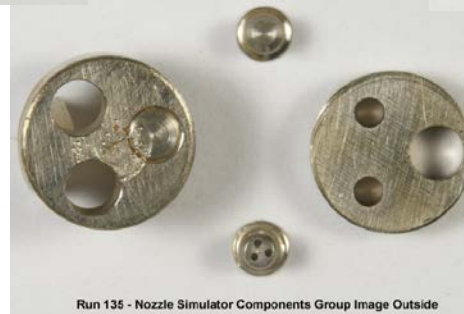
Figure 52 – Comparison of Run 135 (250 ppm Aquarius with 200 ppm Total Dissolved Water) Nozzle Simulator Components To Baseline and 4X Additized Fuel
