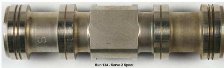
Figure 46 – Comparison of Start and End Program Servo Valve Spools, EDTST-Mode, Baseline and Additized Fuels
