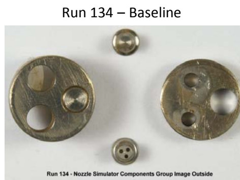
Figure 47 – Comparison of Start and End Program Nozzle Simulator Components, EDTST-Mode, Baseline and Additized Fuels
