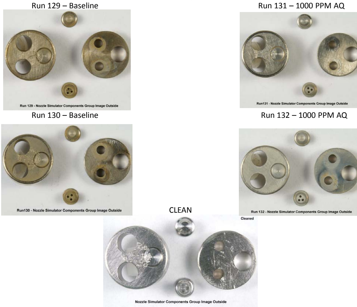
Figure 43 – Comparison of Nozzle Simulator Components, GDTC-Mode, Baseline and Additized Fuels
